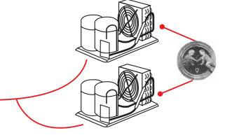
Ventilated refrigeration with uniform temperature: this uniformity is guaranteed by the continuous operation of the vents, or of at least one vent during the defrost stage of the non-refrigerating group. The application of twin systems allows optimal stability of the internal T, as shown by tests carried out in our laboratories (both for positive and negative temperatures); below is an example:
