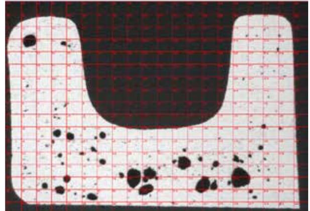
Estimating pore size using live digital reticles
