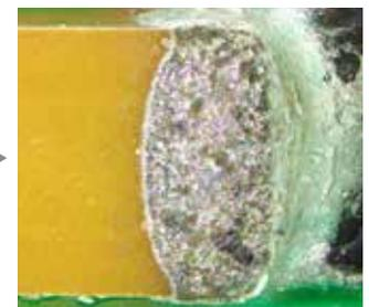
Instant EFI image of a capacitor on a printed circuit board
