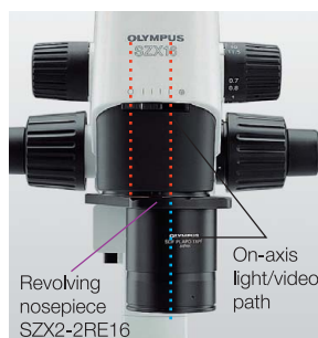
The nosepiece enables vertical observation.
