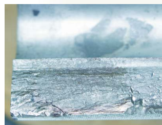
Four-part illumination of surface fracture (metal)
