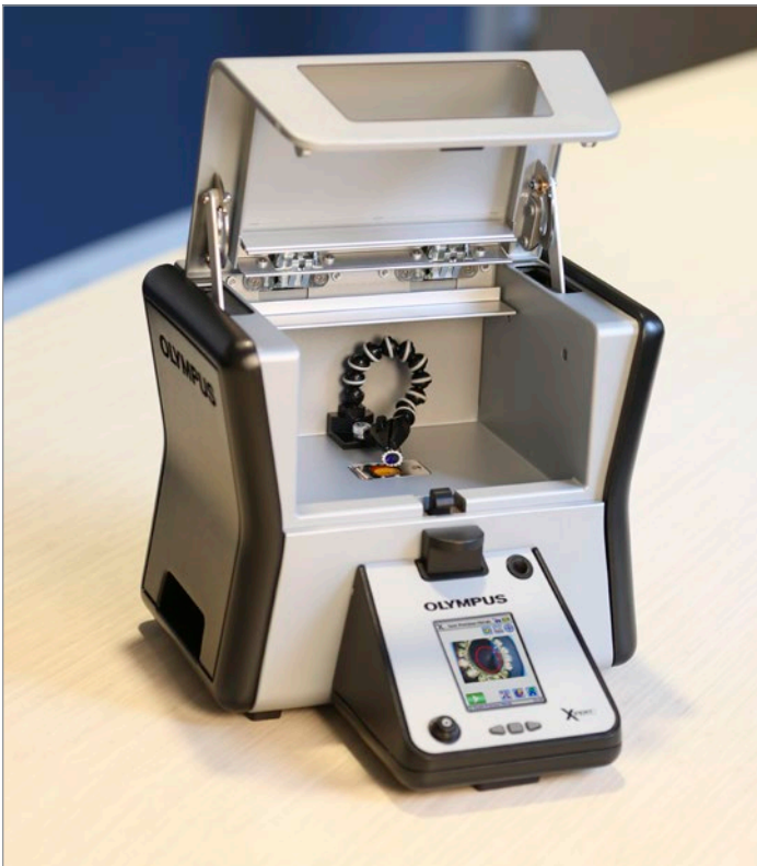
Use small spot collimation for very small objects or for small areas on an object
