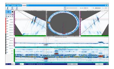
Advanced phased array (PA) inspection technology provides numerous advantages when used in place of radiography testing (RT) to perform piping and vessel weld inspections in compliance with ASME, ISO, and similar fabrication codes. Olympus' PA solution, including WeldSight<sup>™</sup> software, uses 1D phased array probes, TOFD, and DLA\DMA phased array probes for austenitic materials, including cladded piping and dissimilar metal welds.
