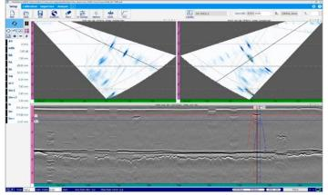
High-speed automated PA and TOFD inspection of wind tower welds in compliance with ISO, AWS, and similar fabrication codes can replace manual probe-in-hand UT scanning. Olympus' automated PA and TOFD solution reliably inspects wind tower bevel designs, including the thickness of transition welds and vertical weld bevels that require unique probe and scan plan considerations.
