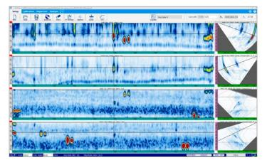
Our PA solution for liquified natural gas (LNG) tank fabrication inspections to API and similar fabrication codes is an advantageous replacement for radiography and conventional UT systems. The solution based on WeldSight<sup>™</sup> software provides improved productivity and real-time analysis, and Olympus' DLA PA probes are effective for the austenitic 9% nickel shell to I625 dissimilar metal welds typical of cryogenic storage tanks.
