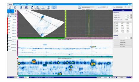
WeldSight software was designed for an efficient workflow and fast training track, leveraging BeamTool software for inspection engineering. Historically, much of the skill and expertise required for advanced phased array inspection was due to complicated software and an inefficient workflow. WeldSight supports high production of compliant, repeatable inspections for the weld fabricator market.
