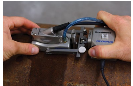
VersaMOUSE and RexoFORM scanners for corrosion inspection.
