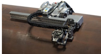
The SteerROVER scanner, when fitted with a motorized raster arm, is a powerful solution for corrosion inspection in remote locations.
