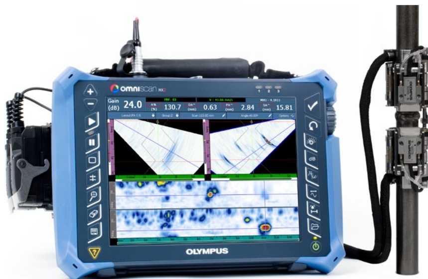
The COBRA scanner on a 0.84 in. pipe with two A15 PA probes with an OmniScan® MX2 16:64 flaw detector displaying two PA groups with sectorial scans and C-scans.
