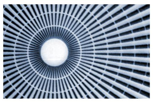
Siemens Star test chart. Even the smallest features of 150 nm lines and spaces can be successfully resolved.
