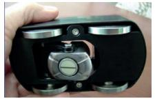
The EZ Scan 4 is a small, single axis linear B-Scan encoder, for use with the T-Gage V DLC, with magnetic wheels and a couplant delivery system. Ideal applications include outside diameter. The scanner comes as standard with a 5Mhz dual transducer spring loaded in two directions, other transducers are also available.storage tank bottom and side walls, flat plates and pipes with a 10cm (4") or greater
